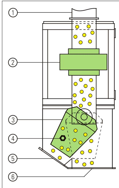
1) Inlet 2) Detection coil 3) Swivel hopper
