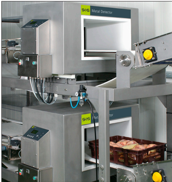
Installation example: GLS metal detectors installed in two production lines to analyze poultry. (old version)
